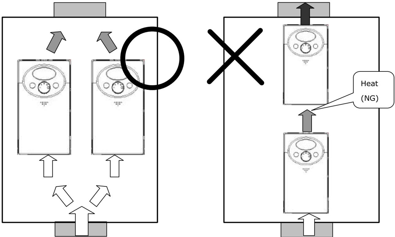
Note : Take caution on proper heat ventilation when installing inverters and fan in a panel.
