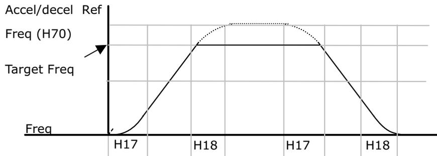
Note: If set target freqs below Max freq, the curve will not be shown completely.
